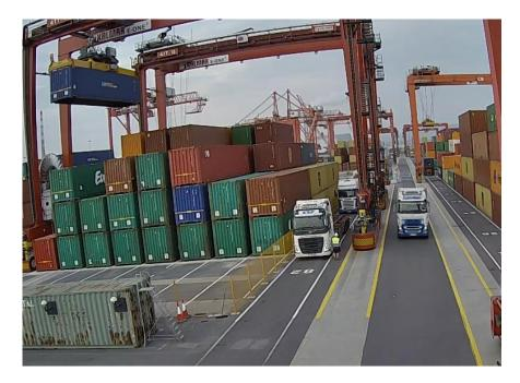
**8.** When the container lands on the trailer, you can inspect the landing, and when correctly on the trailer, signal "thumbs up" to the crane driver, or to any of the trailer lane cameras.
